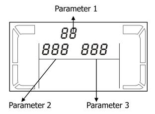
There are three parameters to set up the UPS.
