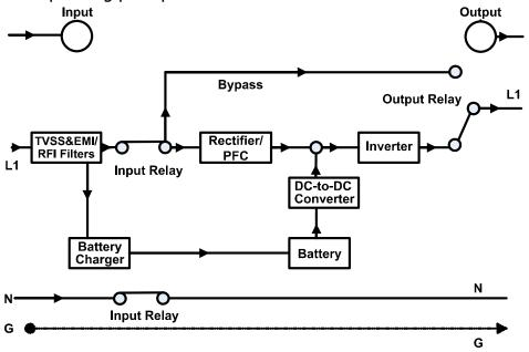
The UPS is composed of mains input, EMI/RFI filters, rectifier/PFC, inverter, battery charger, DC-to-DC converter, battery, dynamic bypass and UPS output.
