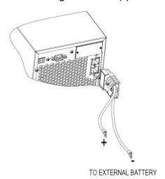
If using rack UPS, the UPS is shipped out from factory without connecting battery wires for safety consideration. Before installing the UPS, please follow below steps to re-connect battery wires first.
